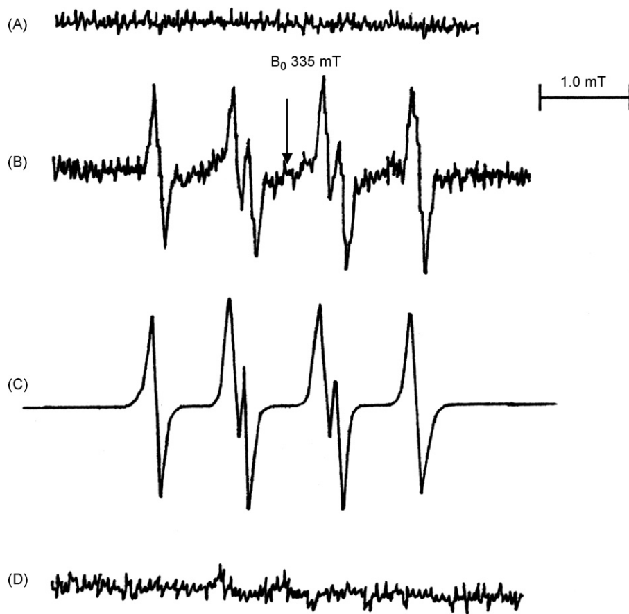
Fig. 8. EPR spectrum generated by irradiation of complex 4 (100 \mu\text{M} ) and DMPO (100 \mu\text{M} ) in air-saturated DMSO solution. (A) in the dark; (B) after 4 min irradiation; (C) the computer simulated EPR spectrum of \text{DMPO-O}_2^{\bullet-} adduct using hfcc values A_N = 1.45 mT, A_H^\beta = 1.32 mT and A_H^\gamma = 0.85 mT and line width used is 0.76 mT; (D) after 4 min irradiation in the presence of SOD. Spectrometer settings—microwave power: 10 mW; modulation amplitude: 0.1 mT; gain level: 6.3 \times 10^3 ; time constant: 0.1 s; scan rate: 4 min, frequency: 9.40 GHz; g_{\text{iso}} : 2.0036.
